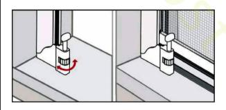
**4.** Only in case of need, fix the rails laterally to the wall.
