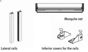
2. The mosquito net is usually installed inside the vain. Depending on the height of the mosquito net it may be necessary to drill the rails and fix them laterally to the wall. Assemble the set of collecting box, rails and inferior covers for the rails, place them in the right place and mark the holes in the box and in the inferior covers. Fix them with the proper fixing screws.
